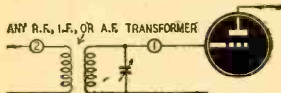
Fig. 4—A quick check method for r.f. coils.
